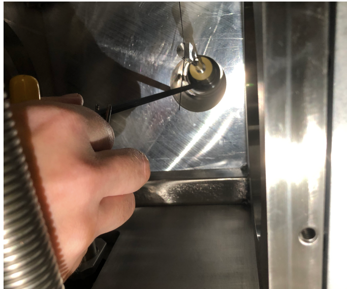
Figure 3: A grounded screwdriver is used to gently scrape the surface of the RPM's insulated base. This was found to alter the RPM's readback noise profile.
