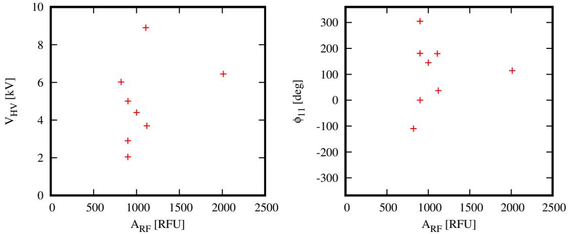
Figure 9: Past operational saved values for the 11 MHz chopper RF amplitude in control system RF units, shown against **Left:** HV plate bias and **Right:** RF phase for different instances of <sup>23</sup>Na<sup>+</sup>.
