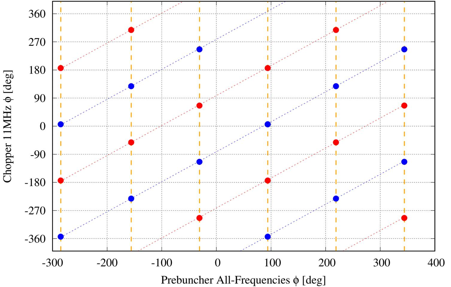
Figure 12: Recorded relationship between prebuncher all frequencies and 11 MHz chopper frequency. Blue dots represent optimum MEBT:RPM5 profile, with sufficient satellite peak separation and overlap to produce a signal on the wire pickup, while red dots show anti-symmetric profiles. Orange dotted lines denote optimum all-frequencies phase for RFQ transmission.
