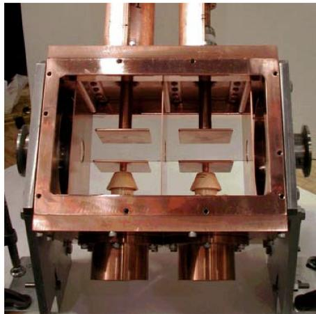
Figure 1: The dual-frequency ISAC chopper on a workbench, obtained from [3].
