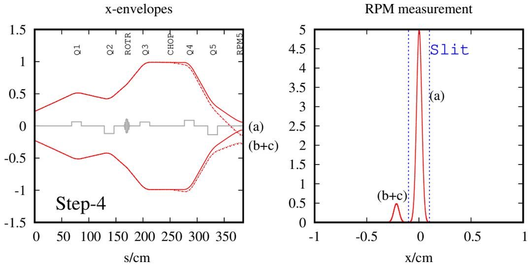
Figure 8: **Left**: Chopper HV plate is set to center beam through chopper slit while causing both satellites to impinge upon pickup wire.
