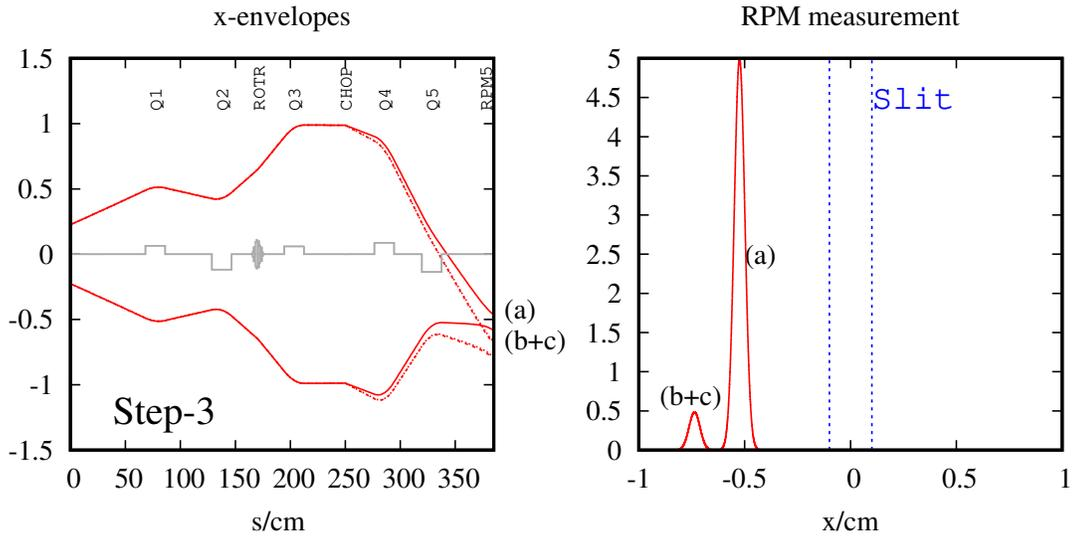
Figure 7: Chopper amplitude adjusted to minimize separation between mean peak and overlapped satellites at MEBT:RPM5 (**Left**), HV plate is off, beam remains uncentered.
