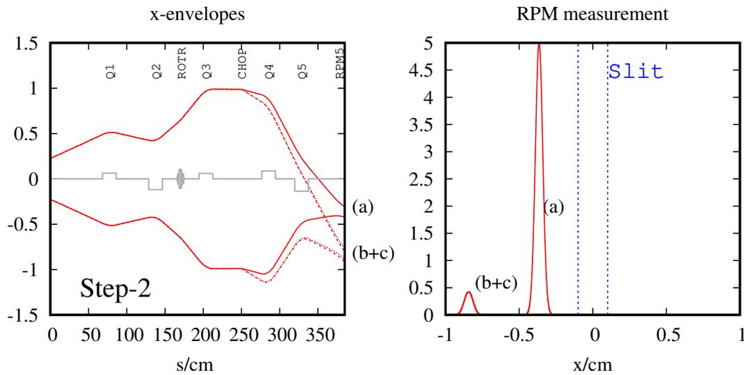
Figure 6: Chopper phase adjusted to overlap both satellites while observed at MEBT:RPM5 (Left), HV plate is off and beam is uncentered.
