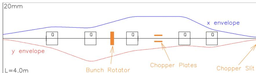
Figure 2: Design beam envelopes[2] in the first 4m of the MEBT section, spanning quadrupoles 1 to 5, terminating at the chopper slit and stripping foil.
