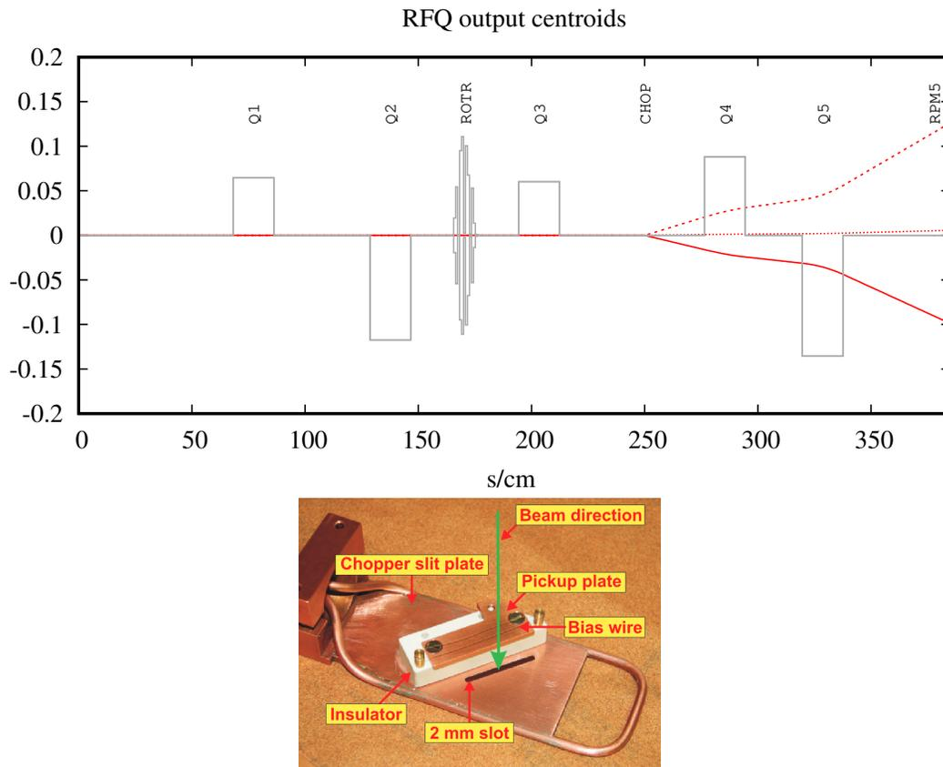
Figure 3: **Top:** TRANSOPTR computed centroids (in cm) through MEBT, assuming perfect input centeredness and deflection through the 11 MHz chopper, which is not optimized. **Bottom:** Image of the MEBT chopper slit, narrowest along the x-axis and widest along y, pictured on a workbench, obtained from [4].
