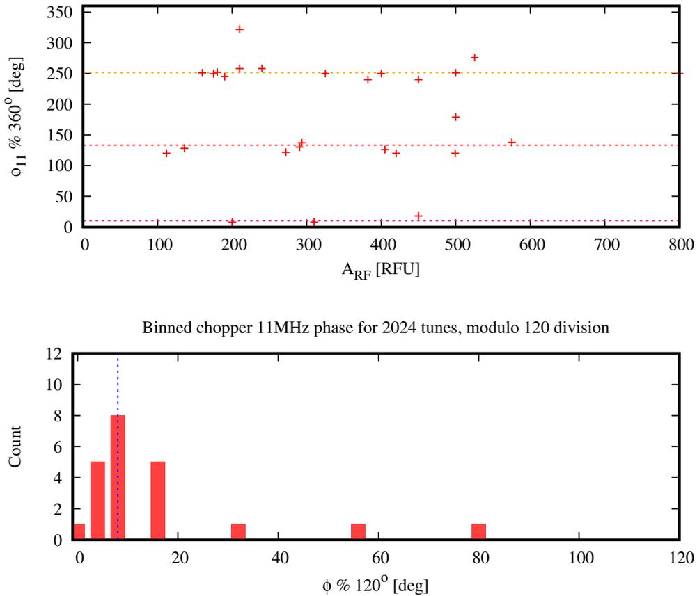
Figure 11: **Top:** 2024 operational saved values for the 11 MHz chopper RF amplitude in control system RF units, shown against **T-Left:** HV plate bias and **T-Right:** RF phase for all accelerated beams. **Bottom:** All chopper 11 MHz phases, after modulo division by 120°, showing a clustering near zero, but with an average remainder of 13.8° after the modulo 120 operation.
