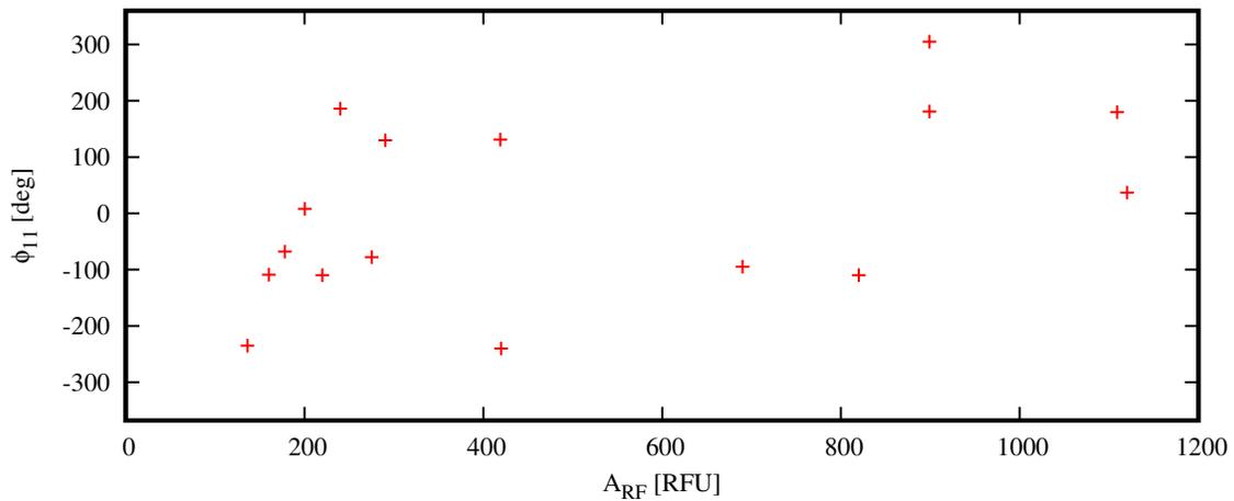
Figure 10: Past operational saved values for the 11 MHz chopper RF amplitude in control system RF units, shown against RF phase, for various beam compositions and charges.
