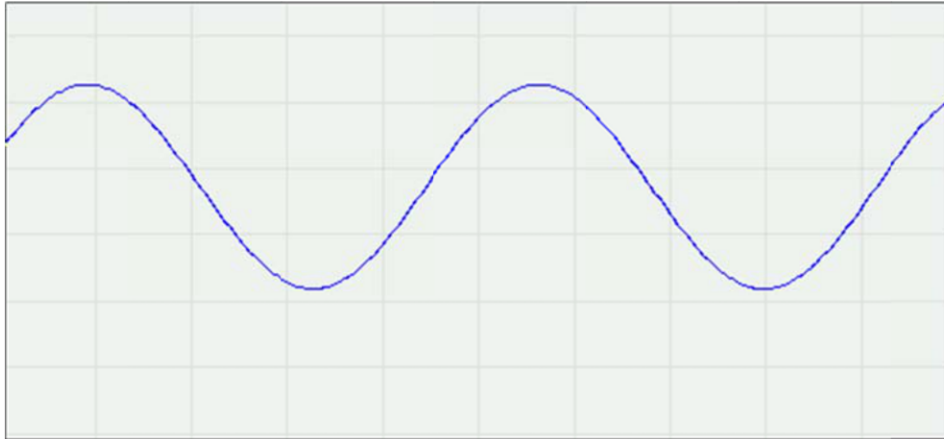
Figure 3: sample 106MHz reflected sine wave from DTL Buncher1, sampled at 2ns/div.
